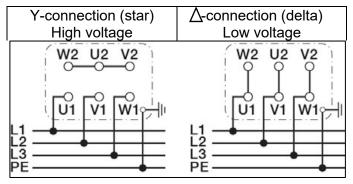
Figure 2 - Connection with six terminals
