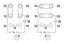
Figure 22 - Single phase motor type GMYC with start capacitor CB and FR protector
