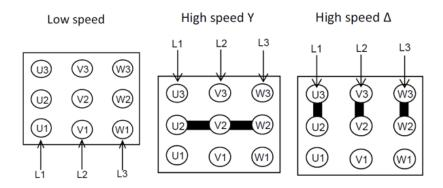
*Figure 26. Three phase dual speed motor with separate windings, like 4/6-pole. Y/D-start at high speed.*
