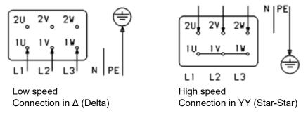
*Figure 4. Three phase dual speed motor with single winding (Dahlander), like 4/2-, 8/4-, 12/6-pole.*
