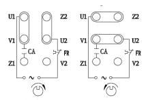
Figure 23 - Single phase motor type GMYY with run capacitor CA and FR protector
