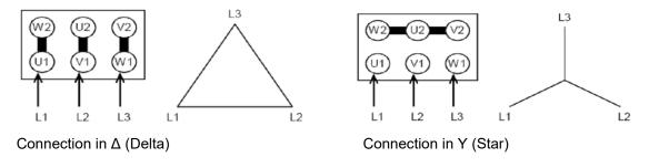
Figure 24. Standard three phase single speed motor.
