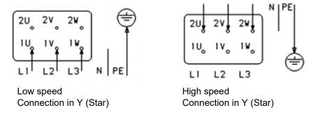
Figure 5. Three phase dual speed motor with separate windings, like 6/4-, 8/6-pole.
