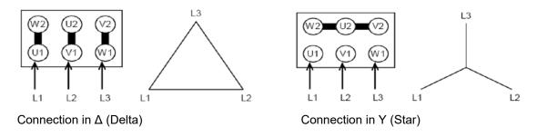
Figure 20. Standard three phase single speed motor.
